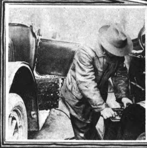
One Way of Quickly Mending Loose Cap on a Country Road,—by Inserting a Small Piece of Match-Stick in the Center, Preventing Further "Skidding."
