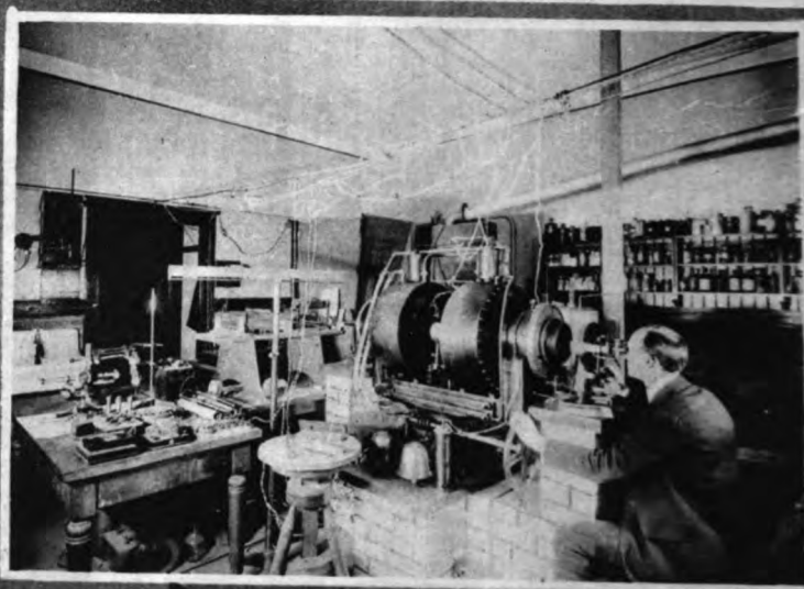
At a Temperature of 573 Degrees Crystalline Quartz Changes Into Another Crystal With a Transfer of Energy During the Process. Remarkable Results Regarding the Temperature Changes Occurring in Crystalline Quartz Have Been Carried Out by Means of the Extremely Powerful Electro-Magnet and Auxiliary Apparatus Shown in the Photo Above.
