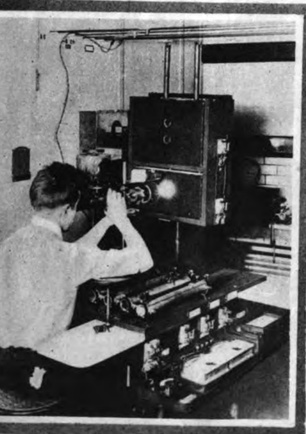
The Photo at the Left Shows One of the Hundred of Different Technical Departments of the Bureau of Standards Laboratories. Here We See One of the Bureau's Engineers Making Researches Into the Heat Liberated by Different Types and Makes of Electric Light Bulbs.
