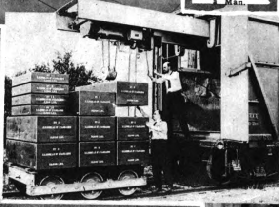
This Giant Testing Machine at the Bureau of Standards Laboratory, Washington, D. C., Can Register With Equal Accuracy, the Power Required to Crush an Egg Shell or That Required to Crumple Up the Strongest Steel Girder. Its pulling Strength Is 1,150,000 Pounds and the Maximum Crushing Power Is 2,300,000 Pounds.
