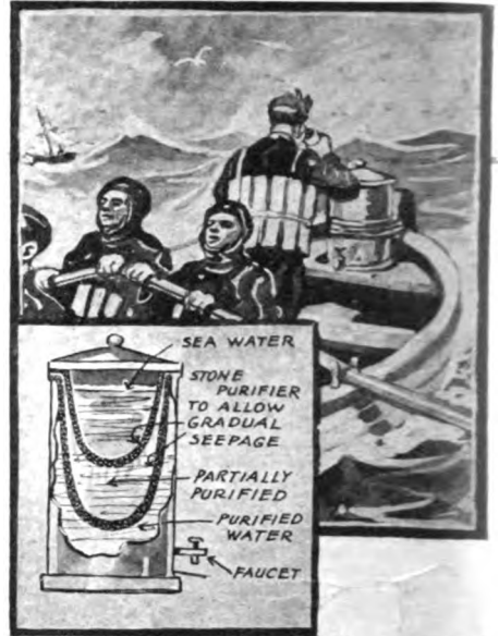
A Simple Water-Purifying Filter, Modeled Somewhat After the Arrangement Here Illustrated, Should Prove Valuable As a Part of Equipment for Life-Boats and in Fact All Vessels Which Make Trips Out to Sea—the Filter After Proper Chemical Treatment of the Salt Water Giving Pure Drinking Water.
