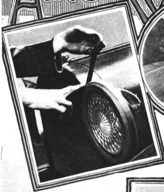
A Stubborn Lamp Rim Will Come Off Easily Without the Damage Done by Tools If Friction Tape Is Wound Around the Rim and Given a Quick Jerk.
