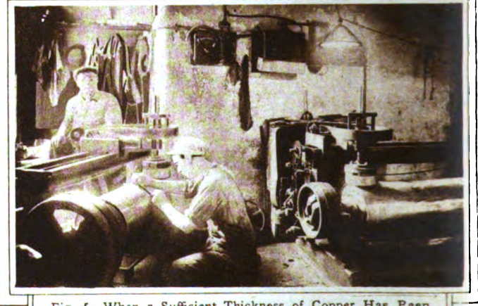
Fig. 5—When a Sufficient Thickness of Copper Has Been Deposited on the Steel Rolls They Are Accurately Turned, Ground and Finally Polished. They Must Have a True and Even Diameter Along Their Entire Length.
