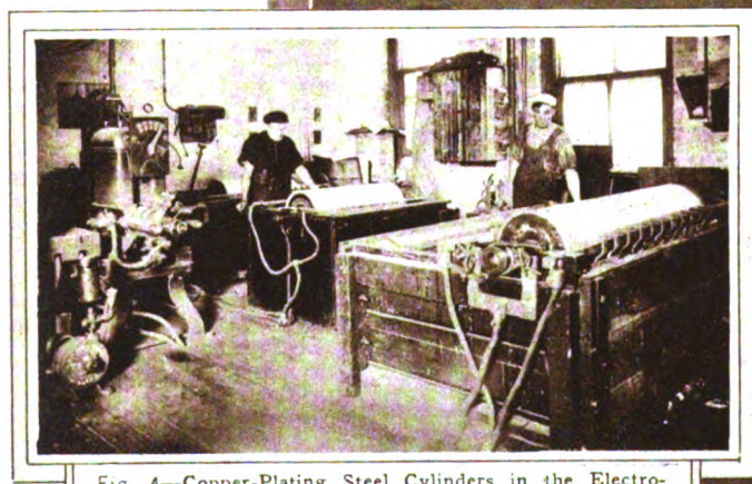
Fig. 4—Copper-Plating Steel Cylinders in the Electro-Plating Room, the Dynamo Supplying the Current for the Process Appearing at the Left. The Copper Is Deposited on the Cylinders Electrolytically.
