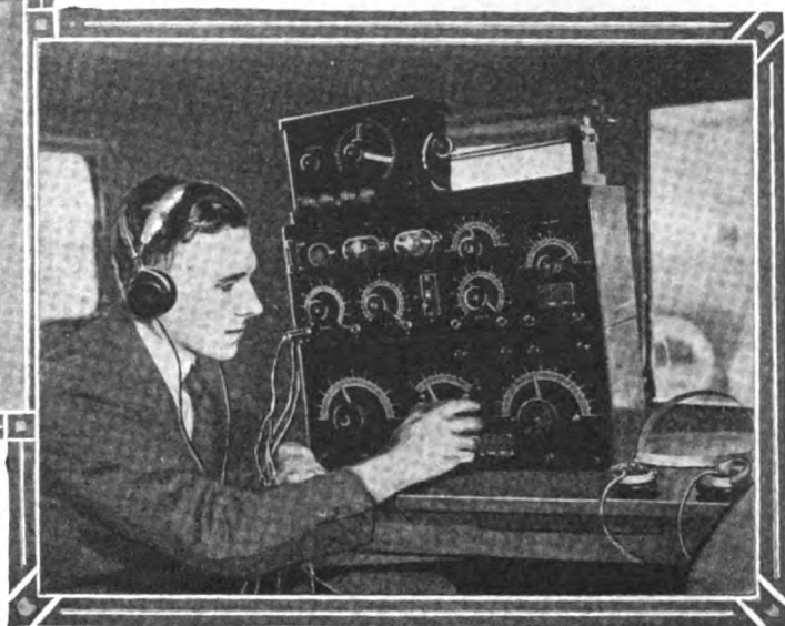
View of Interior of Radio-Equipt Automobile Is Shown Below. Several Stages of Audion Amplification Are Utilized to Boost the Strength of Signals.
