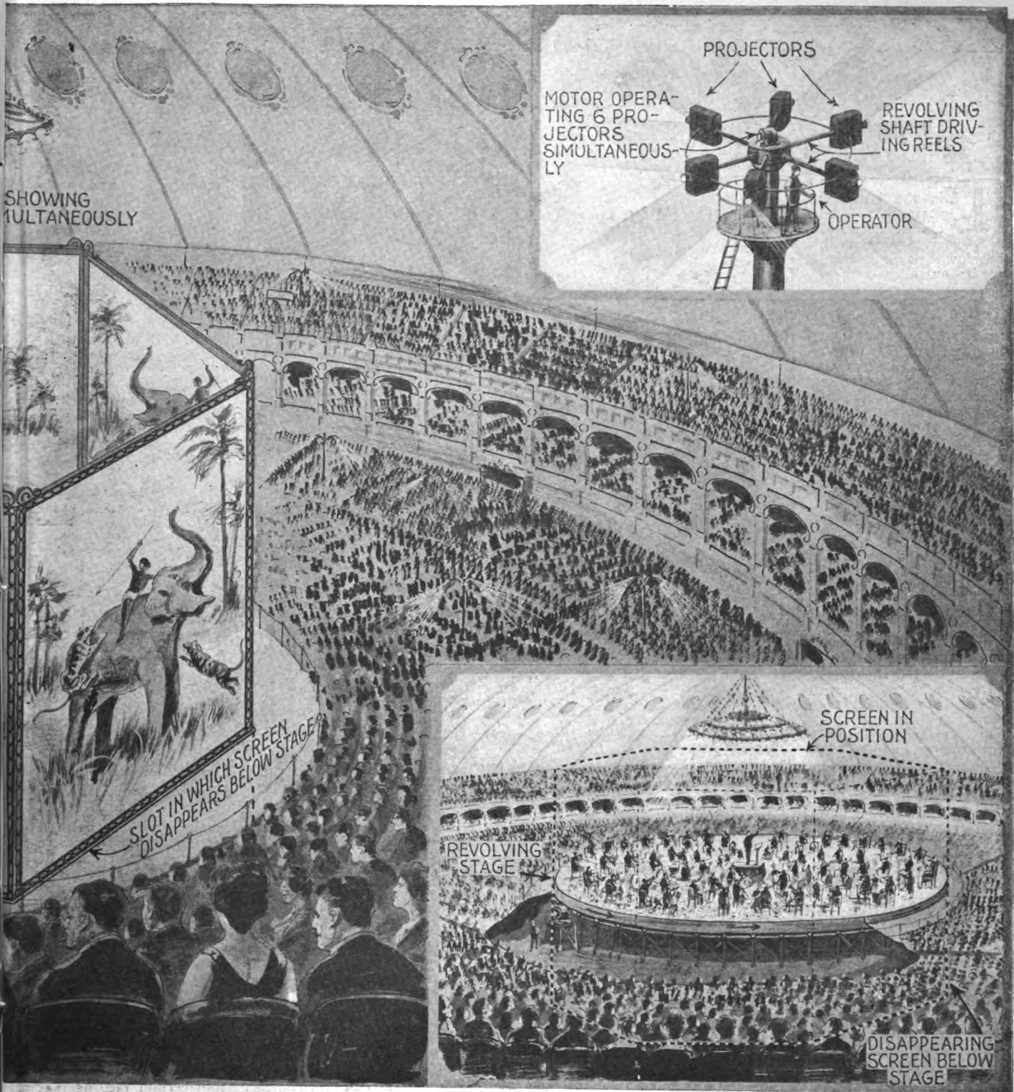
That It Sinks Below the Floor, Unmasking a Revolving Stage Upon Which the Orchestra Is Seated. The Novelty of the Revolving Stage Will Be Appreciated by All Theater-Goers. New Effects Are Provided by Such a Feature, as Is Made Apparent from Our Article. Loud-Talking Telephones Thruout the Auditorium Make It Possible for Everyone to Hear, Even Tho Seated in the Last Row.
