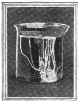
By Dropping a Chemical Seed Into a Clear Transparent Liquid, the Seed Begins to Germinate After a Few Seconds. The Plant Above Resulted From a Crystal of Aluminum Sulfate Dropt In a Water Glass Solution Diluted with Water.
