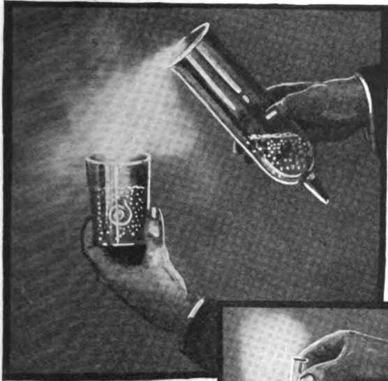
Above: Liquid Air Is Poured Into Water. At First the Globules Float, But as the Nitrogen Evaporates They Become Heavier and Eventually Sink.
