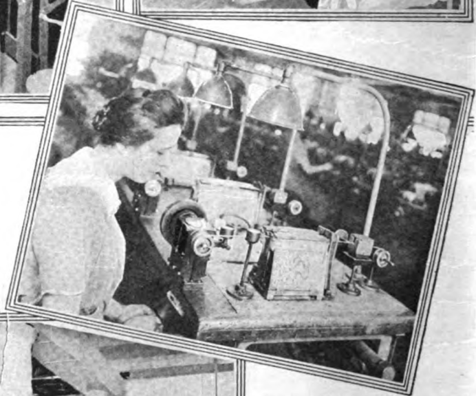
Above:—Drawing Tungsten Down to Finest Proportions, About Four Ten-Thousandths of an Inch or One-Sixteenth of the Size of Fine Human Hair, and Which Cannot Be Seen Except Against a Background of Exactly the Right Color. It Is Used as Filament in the Smallest "Bug" Lamps. The Thread of Tungsten Unwinds From the Spool at Extreme Right, Passes Thru Small Box of Lubricant, Then Thru Gas Furnace Which Has a Diamond Die at Its End Nearest the Operator. The Wire Then Winds on a Receiving Spool and Is Ready to Be Put Into the Tiniest Lamps.
