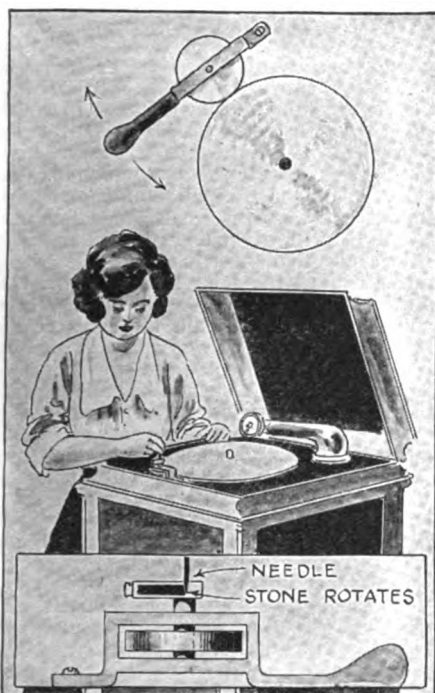
The Phonograph Needle Sharpener is the Latest Invention of Mr. J. G. Hobson. It is a Small Attachment Which Screws to the Top of a Phonograph, and by Means of a Friction Wheel Rotates an Abrasive Stone, Sharpening the Needle in a Jiffy.
