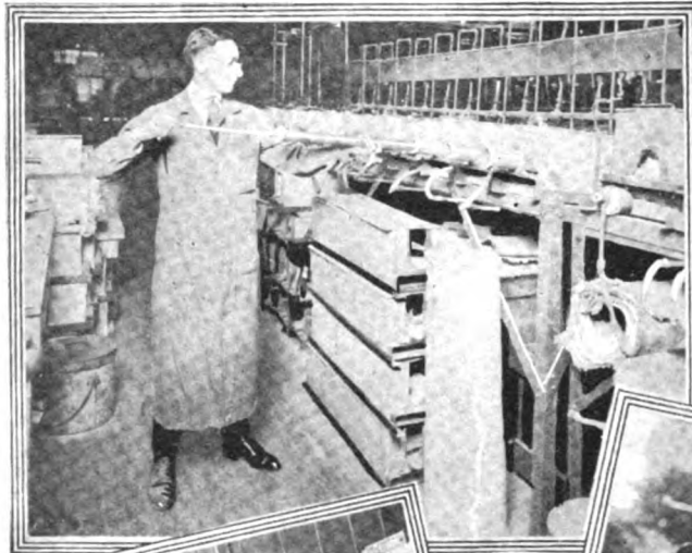
Below We See the Last Process in Using Tungsten in Lamps—Winding the Fine, Tangle Wire on the Lamp Mount by Hand.
