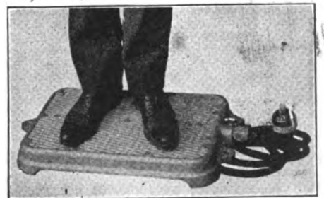
Electric Foot Warmer For Policemen and Others Stationed at Outdoor Posts. The Device Is Thoroughly Water-proof.
