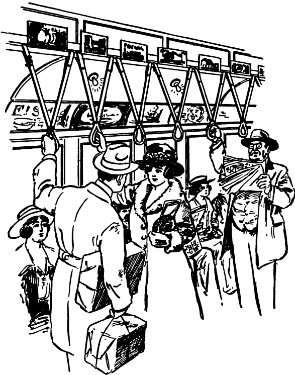
A Novel Invention Is This Idea for Swinging Car Straps. The Strap Swings Only Sidewise and Not Lengthwise of the Car, and at the Top of Each Appears an Advertising Sign.
