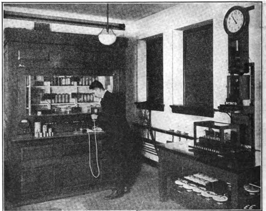
Here We See One of the Government Experts at the Bureau of Standards Laboratories Putting Dry and Other Form of Battery Cells Thru Extensive Tests. The Batteries Can Be Periodically Discharged at Regular Time Intervals by Means of an Automatic Circuit Closer Attached to the Clock at the Right.
