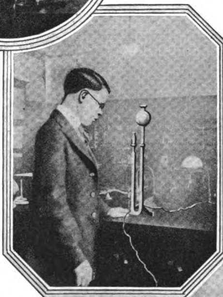
Producing Hydrogen and Oxygen by the Electrolysis of Water.
