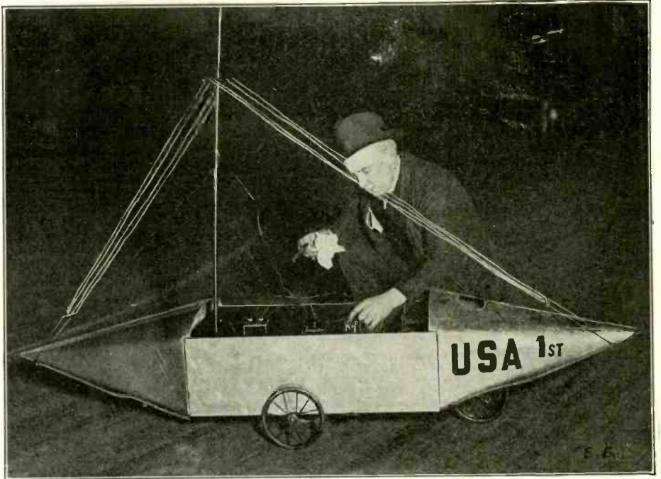
New Radio Controlled Torpedo, Devised by a New York Inventor, Mr. E. F. Galvin. The Radio Waves Are Intercepted by the Antenna Wires Supported from the Mast.
