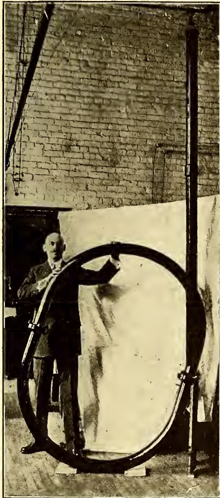
Prof. Goddard and His "Vacuum" Pipe, by Which Tests Simulating Those in the Upper Atmosphere Were Made With His New Rocket.
