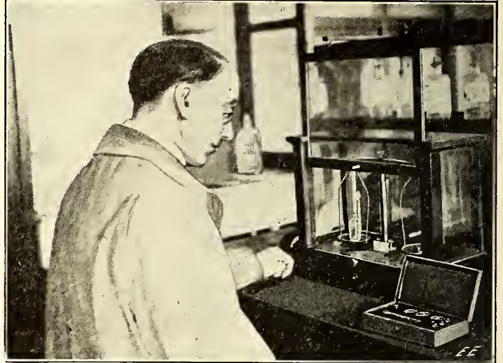
Making Westphal Balance Test for Percentage of Alcohol.
