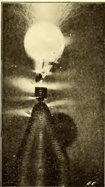
Many Spectacular and Beautiful Effects Are Obtainable When a Large Incandescent Lamp Is Lighted by an Oudin Coil. This Experiment Shows a 250 Watt Lamp Being Illuminated on a 200,000 Volt Oudin Coil by a Unipolar Discharge.
