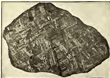
Slice of Kingston Meteorite Showing Widmanstätten Figures. This Meteorite Fell in New Mexico. The Figures Are Obtained by Polishing and Then Etching the Metal by Means of a Weak Acid.
