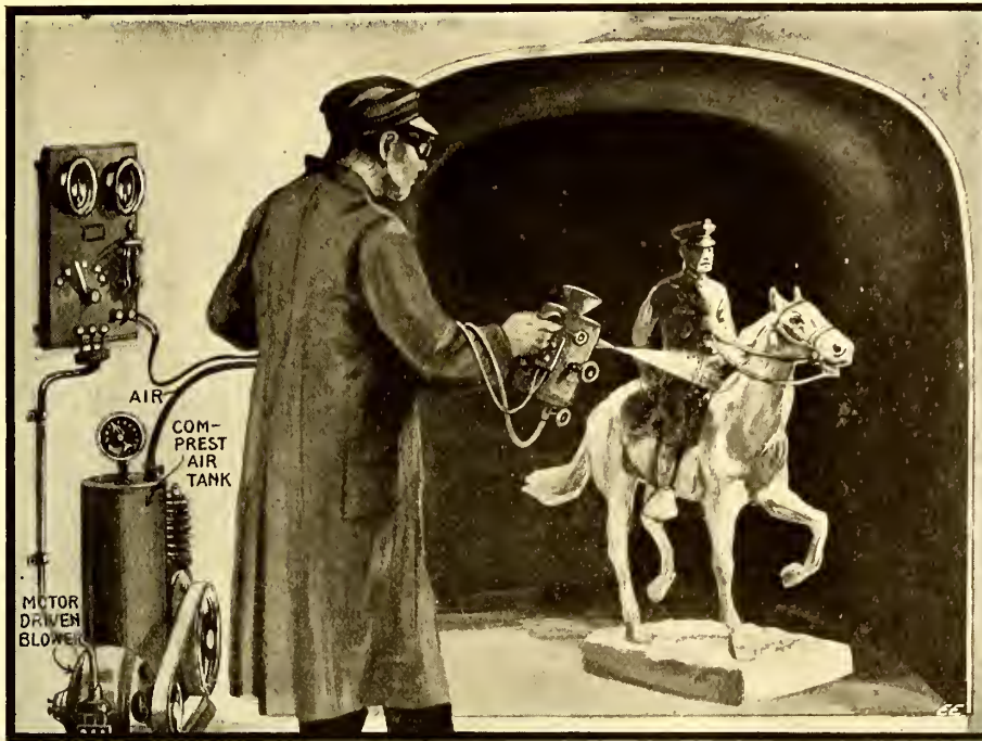
The Wonderful New Compress Air System of Plating Any Object with Metal to Any Desired Thickness. The Metal to be Plated on to the Object is Placed in the Hopper of the Electric Arc Heater, Whence it Descends Slowly into the Arc, Where it is Instantly Melted and Then Blown by Compress Air Thru a Suitable Nozzle onto the Object to be Plated.
