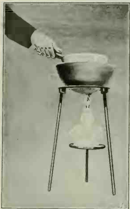
Fig. 1. Apparatus Used In Making Test for Butter and Oleomargarin or Renovated Butter.
