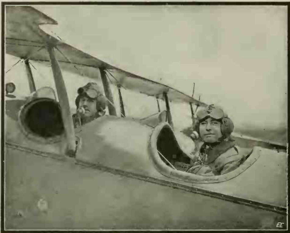
U. S. Army Airplane Pilot and Observer Equipt with Wireless Telephone Sets for Transmitting as well as Receiving Speech. These Sets Are Provided with a Change-over Switch Which Permits the Instruments to Be Utilized as a Regular Telephone Between the Two Birdmen.
