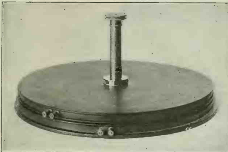
Tesla's Static Eliminator, Patented and Used by Him over Twenty Years Ago. It Will Be Fully Described in an Early Issue of the Electrical Experimenter
