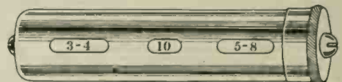
A Useful Computer for Machinists and Experimenters. It Shows the Size of Drill for Any Tap Instantly.
