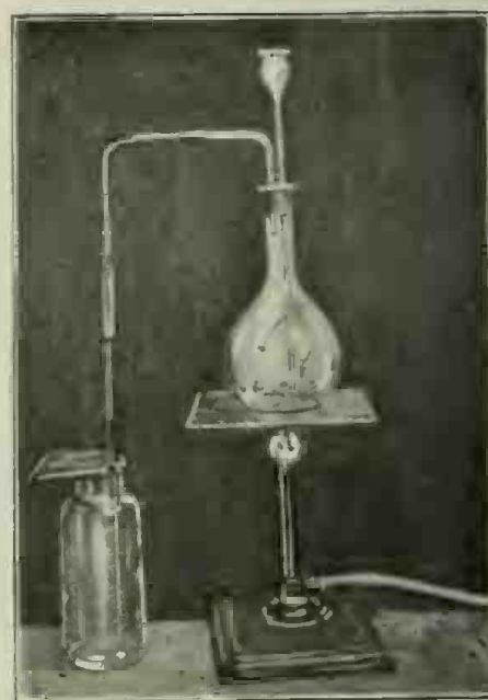
Fig. 136. Apparatus for the Dry Collection of Chlorin Gas by the Displacement of Air. Height of Gas in Bottle Is Seen by Its Greenish Color.
