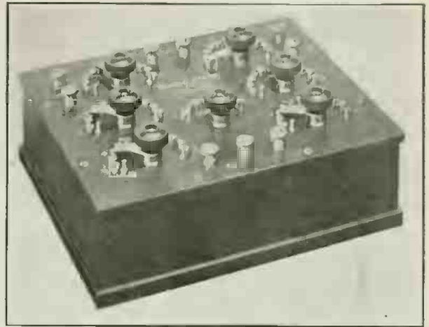
New Radio Frequency Decade Bridge Suitable for Measuring Inductance, Capacity and Resistance. Fig. 2.
