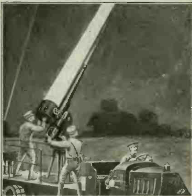
English Anti-Aircraft Guns Used in the Aerial Defense of London Have Been Fitted With Searchlights to Increase the Accuracy and Rapidly of Fire, This Unit Being Mounted on a Motor Truck.
