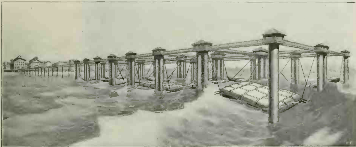
The Latest Idea in Wave Motors—It Comprises an Extended Series of Buoyant Tanks or "Floats." Each Float Rising and Falling with the Waves and Serving to Compress Air. The Comprest Air Drives a Pneumatic Motor Connected to a Dynamo, Thus Producing Free Electricity From the Ocean Waves.
