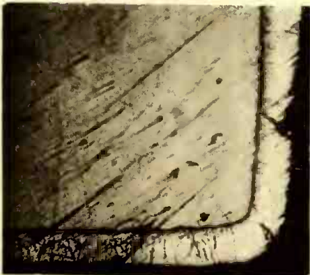
Microphotograph of Electrically Sherardized Steel, Which Is Rust Resisting. The Black Line Indicates the Minute Joint Thickness Between the Metal and Coating—It Having Been Magnified 150 Times.
