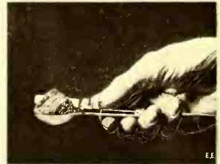
A New Measuring Spoon Which Saves Much Time and Many Poor Mixtures. It Always Levels Off the Spoon Even and Is Graduated as Indicated.
