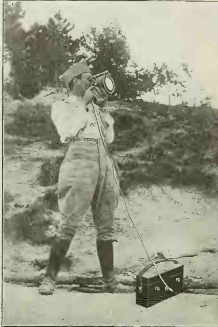
The French Army Has Recently Perfected a Miniature Searchlight and Telescope for Signaling To and From Aircraft in Daylight, as Well as at Night. It Has a Range of Two Miles in Broad Daylight.
