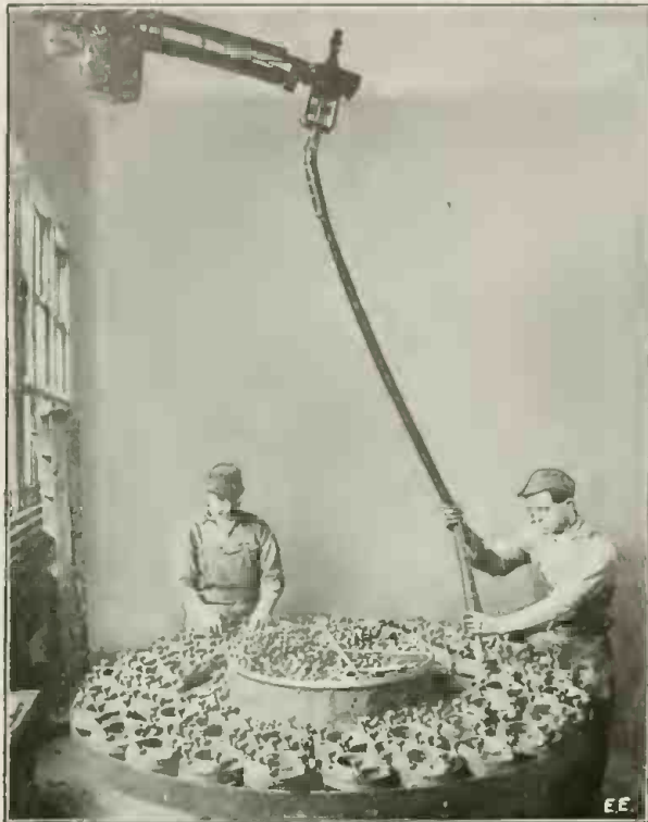
The Nuttiest Job Agoing. One Operative with This Electric Nut-Screwing Device Can Screw Down Nuts at the Rate of 100 a Minute at a Cost of 1 Cent an Hour.
