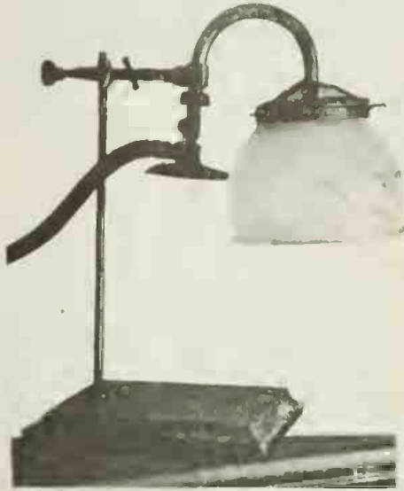
A Quickly Made Desk Lamp Constructed from a Ring Stand, a Bunsen Burner, Goose Neck, Mantle and Globe.
