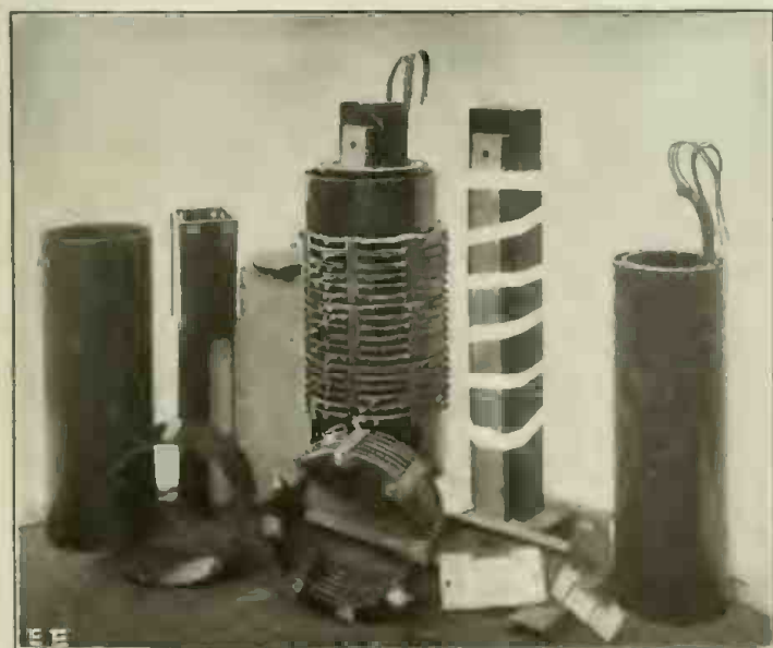
New Core Type Transformers with Concentrically Arranged High and Low Tension Windings.
