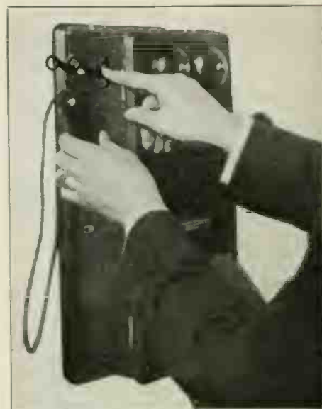
This "Battery Saver" Telephone Attachment Permits One to Listen In on a Line Without Wasting Battery Current.
