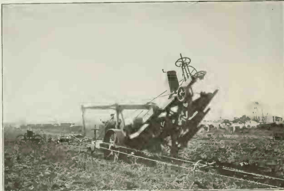
The Teuton Tillers of the Soil Make Extensive Use of Electrically Operated Plows, One of Which is Illustrated Above. Current Is Supplied the Motor Thru a Trolley Wire.
