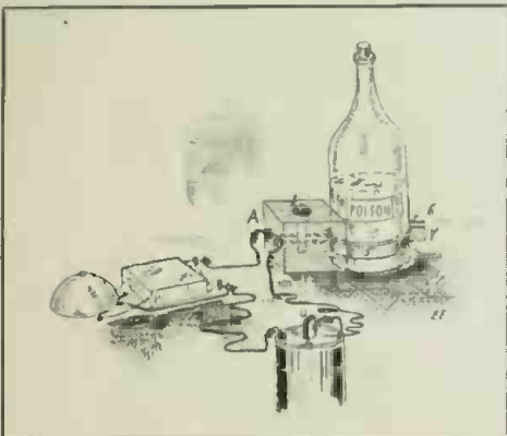
When the Poison Bottle is Removed From the Contact Strips, They Spring Together, Closing an Alarm Bell Circuit.
