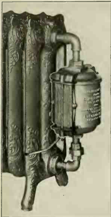
This Induction Electric Water Heater is Intended for Use on Radiators, etc. It Involves the Use of a Coil Thru Which A. C. Passes, Which Causes a Water Heating Member to Become Heated by the Current Induced in It.
