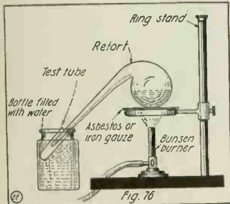
Method of Setting Up Retort, Bunsen Burner, Condenser, Etc., in Experiment No. 82.
