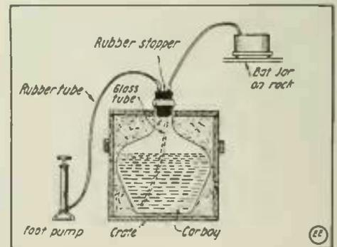
Method Whereby Battery Electrolyte Can Be Pumped by Compressed Air from Carboys into Cells.
