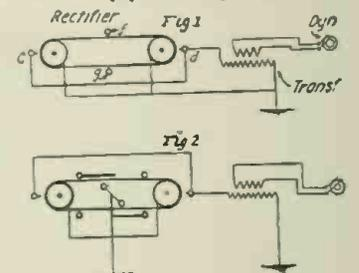
The two metal rolls are grounded and as the paper travels around, it carries negative charges from "c" and "d" to "f" and "g." The apparatus in Fig. 2 is for producing positive electricity.
