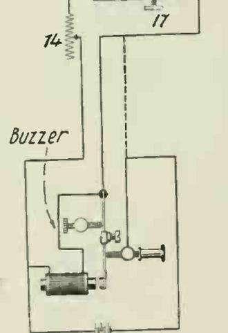
The apparatus in question consists of a telephone receiver connected with a circuit comprising a battery and a rapidly interrupted switch or contact, such as a buzzer.
