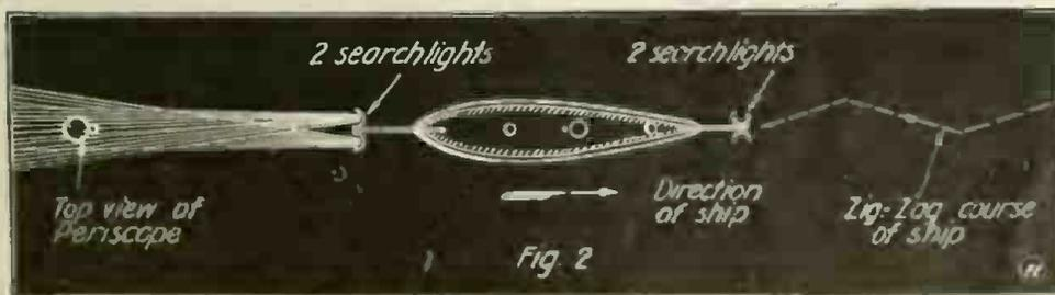
From the Ship's Position As Shown in Fig. 1 It Now Swings About—Still Keeping the Searchlights On the Enemy's Periscope—Thereby Presenting Its Narrowest Part to a Possible Torpedo. Then By Zig-Zagging, the Attacked Steamer Can Escape.
