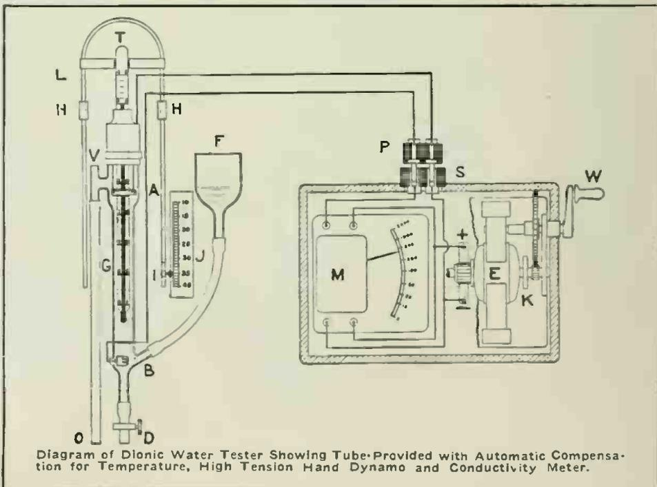
Diagram of Dionic Water Tester Showing Tube Provided with Automatic Compensation for Temperature, High Tension Hand Dynamo and Conductivity Meter.
