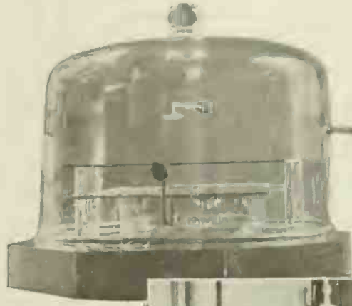
Fig. 3 (At Left). Jar for Making 11-inch Partly Transparent Mirrors. The Cathode is at the Bottom and Consists of a Thin Sheet of Gold or Platinum-iridium Alloy. The Glass Plate to be Coated is in a Plane Parallel to the Cathode.
