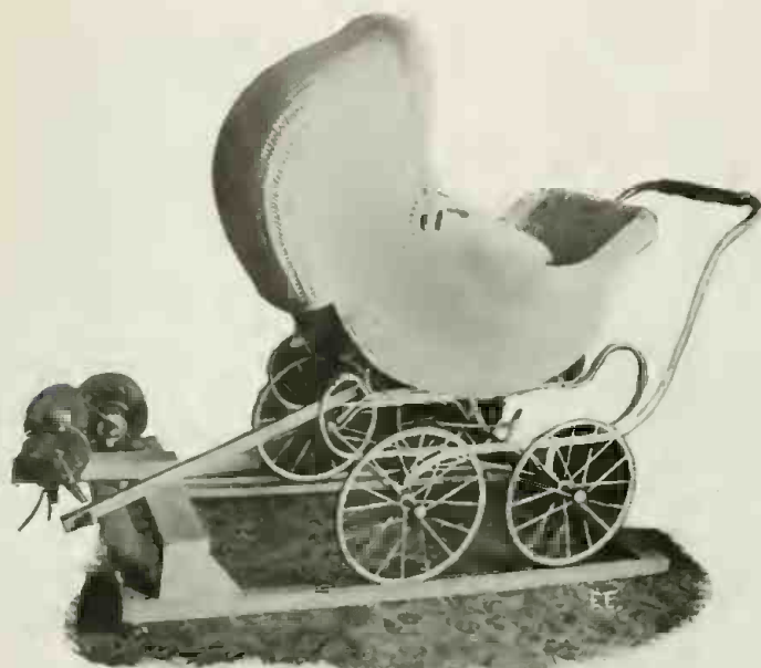
A Chicago Genius Has Evolved a Clever Combination—a Baby Carriage Plus an Electric Motor and Part of a Small Grinder Reduction Gear. Result—No More Pushing the Baby Carriage Back and Forth. We'll Bet His Wife is a Suffragette!
