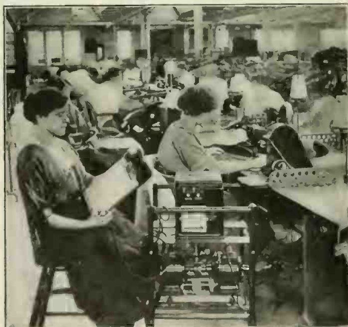
Here We See a Portable "Productograph." Connected to Each Machine It Enables the Young Lady in the Foreground to Readily Keep an Exact Record of Each Employee's Output.
