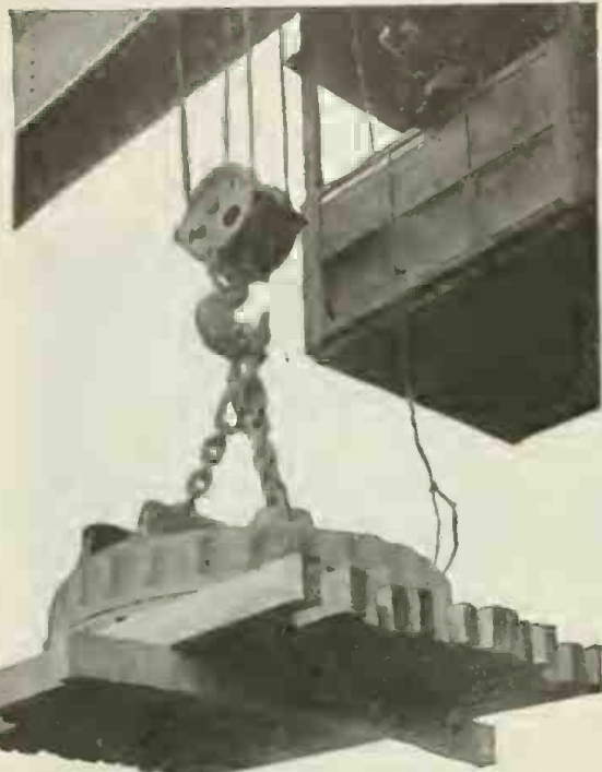
The Crucible Steel Company Have in Use at Their Pittsburgh Plant This Gigantic 62-inch Electro-magnet. It Can Lift 4½ Tons of Steel Bars and the Trip of a Switch Releases the Entire Load Instantly. This Class of Work Spells "Economy" in Big Letters and Foundries Everywhere Are Rapidly Awakening to the Fact.
