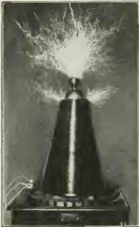
Fig. 1. View of the Strong Conical Oudin High Frequency Coil Delivering a Veritable Tree of Sparks Several Feet In Length.
