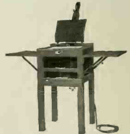
Electrically Illuminated Photograph Printer Equipt with Automatic Switch Actuated By Printing Frame.
