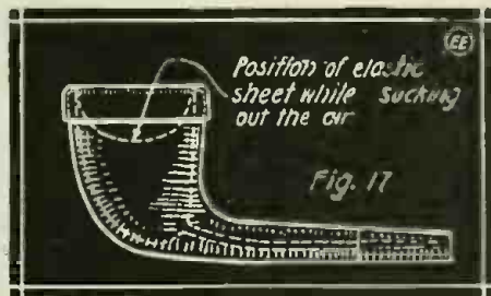
Removing the Air Within a Pipe Bowl by Sucking In Thru Stem Allows the Pressure of the Air to Push Elastic Diaphragm Inward.
