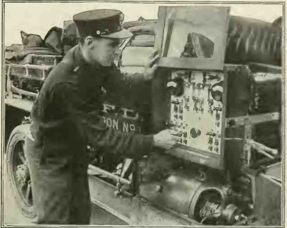
Los Angeles, Cal., Boasts of Having One of the Most Complete Electric Fire-fighting Trucks in the United States. The Equipment Comprises Five Powerful Searchlights Which Are Supplied with Power from Either a Large Storage Battery or the Dynamo Shown in the Picture.
