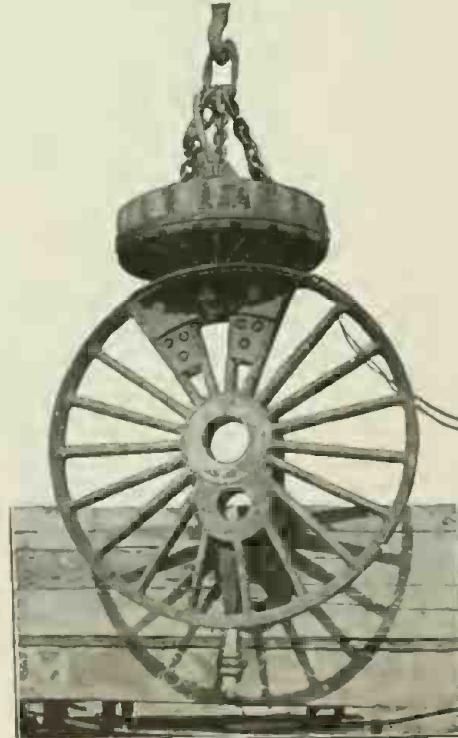
43-Inch Magnet Lifting a Locomotive Drive Wheel at the West Milwaukee Shop of the C. M. & St. Paul Railway. Another Instance of What the Lifting Magnet Is Capable of Doing.
