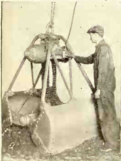
Fig. 1. Small Grab Bucket Opened and Closed by Electric Motor Mounted Directly on Same.
