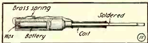
Electro-magnetic Screw Driver Having Flash-light Battery in Handle.
