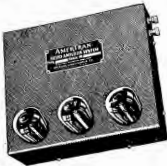
*AmerTran Push-Pull Amplifier Type 2-AP. Complete 2 stage audio amplifier with first stage AmerTran DeLuxe for XU227 AC and second stage AmerTran Push-Pull for two 171 or 210 power tubes. Operates with 450 volt AmerTran Hi-Power Box. Price east of Rockies—less tubes—$80.00.
