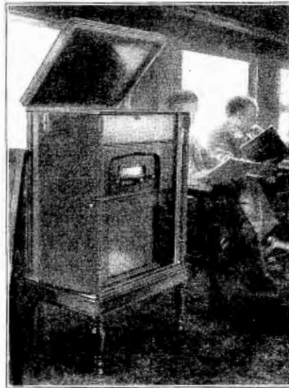
Fig. 5. The latest in radio broadcast receiving equipment on railway trains as installed in a compartment-observation-library car of the Canadian National Railways. The receiver is a standard all-electric ten tube set with phonograph combination and dynamic speaker. Alternating current for the operation of the receiver is supplied by a motor generator set which takes direct current from the car lighting system at 32 volts and converts it into alternating current at 110 volts 60 cycles
