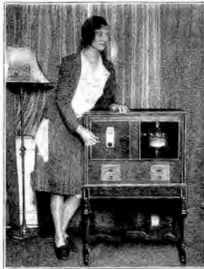
Photograph K illustrates the latest Jenkins experimental console containing a model 200 radiovisor mechanism with the special Jenkins television receiver and loud speaker
