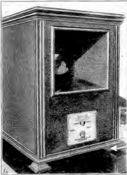
Photo I shows a front view of the large Jenkins radiovisor showing the shadowbox and the control panel. This type of radiovisor has been seen by fans at the radio shows during the latter part of 1929. It is intended more for home entertainment than for experimental purposes
