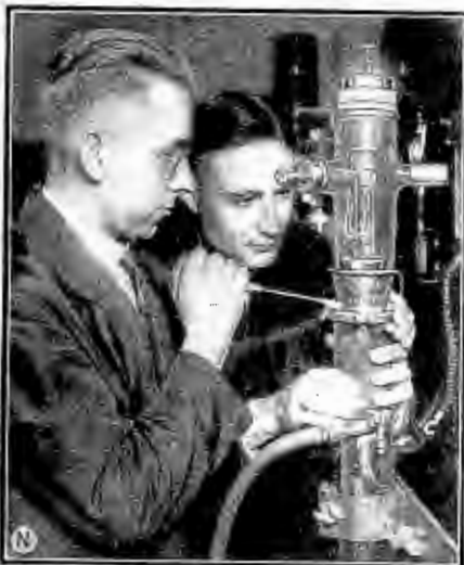
With the erection of the giant radio broadcast station, the "Deutschlandsender," at Seesen, Germany, bids fair to rank with the radio centers of the universe. The one at Seesen is of world-wide proportions. Photo N shows the water-cooled type of transmitting tubes used. P. & A. Photo
