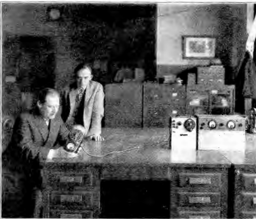
Fig. 8. In this photograph at the right are the radio set which transmits a radio wave and preserves the echo, and the altimeter developed by E. F. W. Alexanderson, consulting engineer of the General Electric Company. Dr. Alexanderson is holding the memory meter on which the altitude is recorded. With him is his assistant, S. P. Nixdorff
