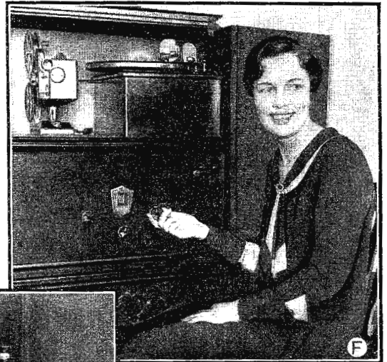
Photo F. By the skill of engineers of the Sonora Products Corp. of Chicago, the first amateur talking pictures are made possible. The 16mm motion picture film is used in connection with a blank phonograph record and by means of a combination hook-up the picture is synchronized in sound. In projection the record is placed on an ordinary phonograph timed with the projector and the results are—home talking movies. Photo shows Miss Doris Sass operating a home "talkie" movie. Wide World Photo
