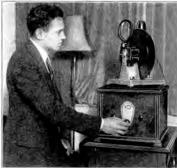
Photo B shows the Jenkins model 100 radiovisor with the special Jenkins television receiver being operated by H. G. Miller, who designed the receiver
