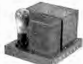
Lincoln DeLuxe 10-B supplies correct B voltages for Lincoln DeLuxe 10; also 60 mills, 150 volts for field of Dynamic Speaker.
