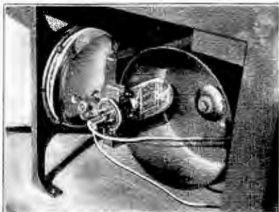
In Photo J may be seen the mechanism of the radiovisor, showing the scanning drum, television lamp and magnifying lens. The synchronous motor and the selector disc do not appear in this picture
