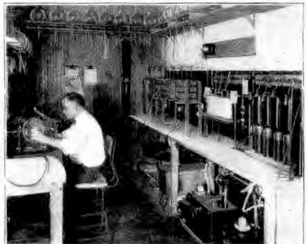
Fig. 3. Separation and purification of rare gases for gas type rectifier tubes
