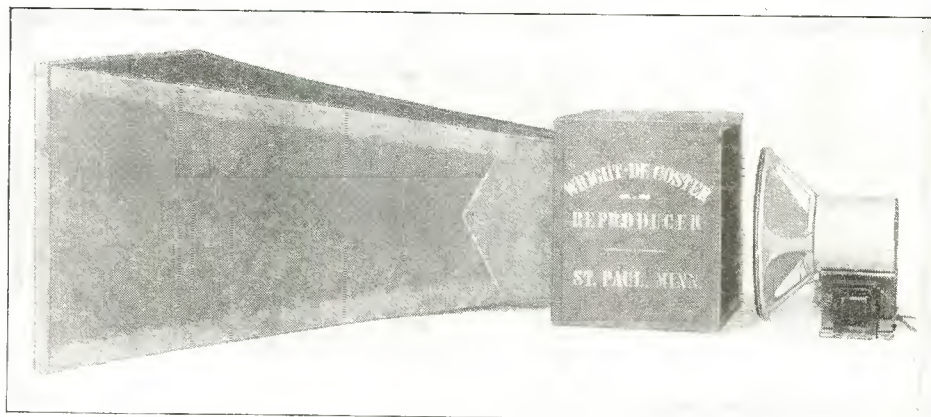
Fig. 10. In this photograph the dynamic speaker made by Wright-DeCoster is shown separately from the horn which was recently tested in our laboratory
