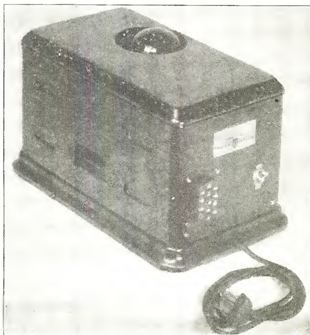
Fig. 4. This photograph shows the power supply which is used separately with the Tyrman 72
