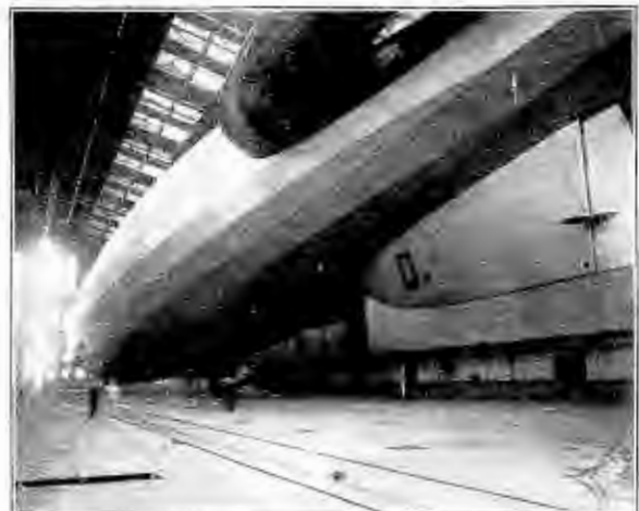
A view of the huge "Graf Zeppelin," taken in the Naval Hangar at Lakehurst, N. J., plainly showing the damaged left stabilizer that slowed up the air voyage and which might have proved disastrous.
