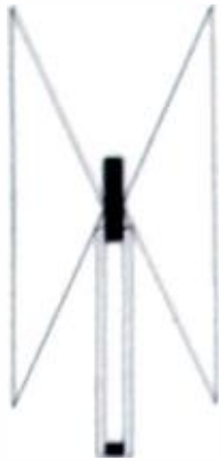
SECTION of the New Acme FREE-EDGE CONE Loud Speaker, showing the two free-edge cones
