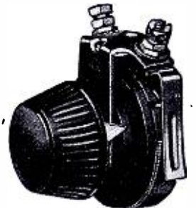
The closely wound, fine resistance wire is prevented from slipping or wearing out of true by a bronze spring. Thus smooth, quiet control is assured either advancing or decreasing the potential.
