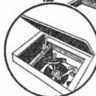
Insert shows top of instrument with automatic record changer.
