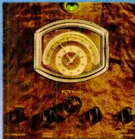
Selector Dial. Note Band Spreader (small pointer operating on white inner scale).
