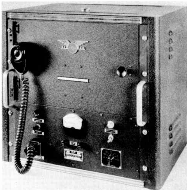
Fig. 5. Aerocom aeronautical base station transmitter.
