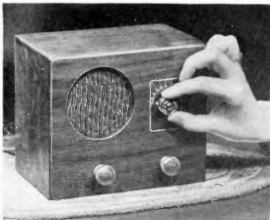
The author built the cabinet of \frac{3}{8} " thick white wood
