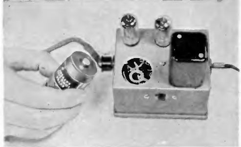
Positive contact of the "A" battery is made to a lug soldered to one of the lugs on the switch. The minus connection is made by contact with cabinet
