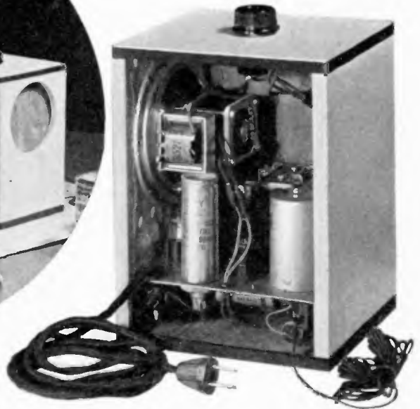
Putting finishing touches on the cabinet. At the right is a rear view of the completed set. The knob on the top is the receiver's volume control
