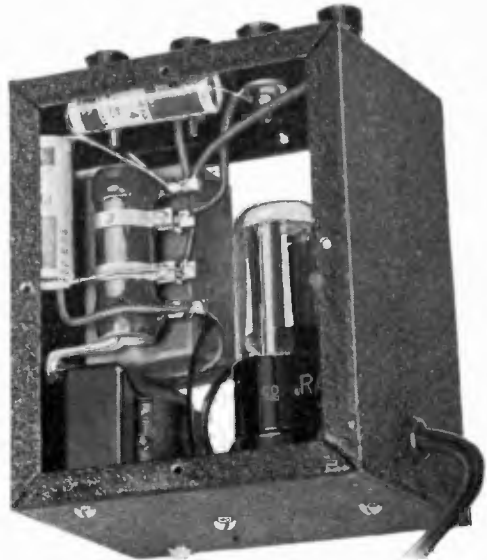
This photograph will help you assemble the outfit in its steel cabinet
