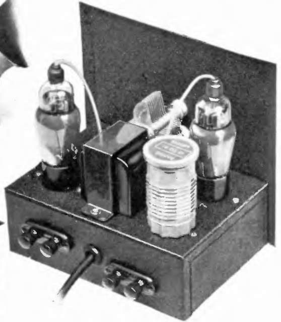
Mount tubes, tuning condenser, transformer, and plug-in coil atop the chassis; other parts (left) below it
