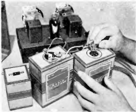
Three new-style batteries are used to power the receiver. The plug-in-type connectors save time
