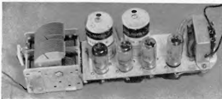
Top view of radio chassis. Left to right, trimmer and tuning condensers, three 1T4 tubes, one 3Q4 tube, and output transformer
