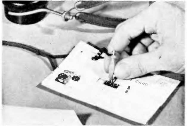
The letter radio can be mailed out of town for six cents. It is tuned by moving a spring clip from one coil tap to another
