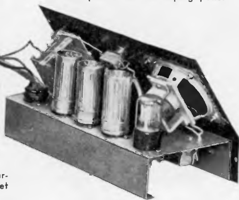
Keep tuned as you ride with this receiver. Note below how tubes are mounted on aluminum chassis, and the speaker on the sloping panel
