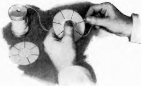
The wire goes over and under the form ribs
