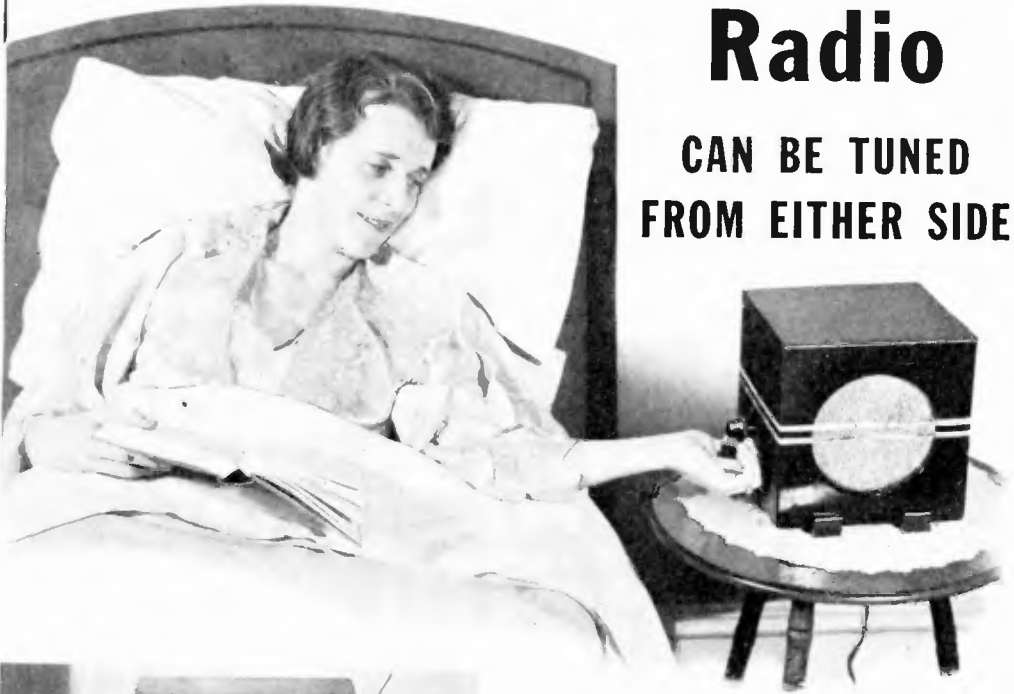
At the flip of a switch, either of two pairs of controls on opposite sides of this twin-bed radio will tune and regulate the receiver
