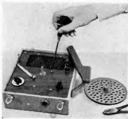
Above, the top of the control panel, with the record turntable removed. This gives a view of the opening for the speaker, in the rear, and the speed regulator under the turntable
