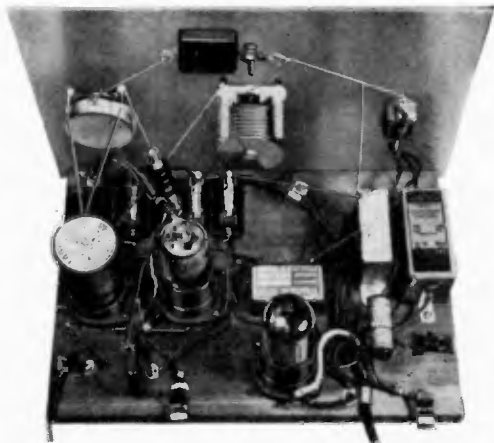
How the two-tube set on page 10 should look after adding a stage of audio amplification
