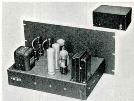
PRE-AMPLIFIER CHASSIS AND ASSEMBLY Chassis: 17" x 10" x 3"; Case: 19" x 13" x 8 3/4"
