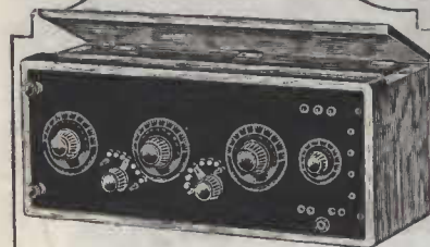
This illustration shows the Three Circuit Tuner and Detector completely assembled in the handsome cabinet.
