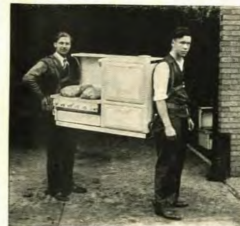
AT LEFT: Illustrating the ease with which a 450-pound refrigerator can be carried up a stairway. One or two men, depending on the weight, can hook in with Muvafast to the rear cuffs on the WRAP-JACK straps and maneuver the refrigerator with the same ease as the man in front. Takes less than two and one-half minutes to lock the WRAP-JACK on refrigerators.
