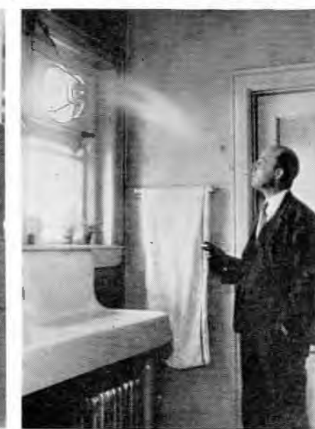
4. Incense or smoke offers the ideal way to demonstrate how soiled air heads for the kitchen window and out.
