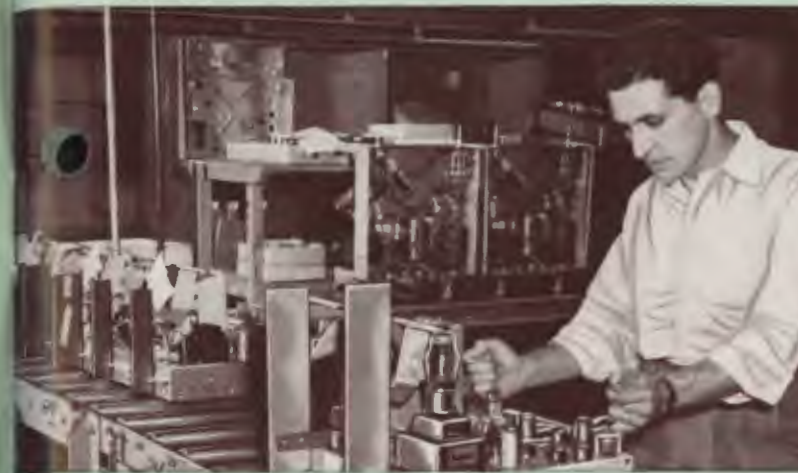
"SHAKE TABLE" TEST checks the stability of connections with an extremely rough "ride" on vibrations more violent than in normal usage, movement or transportation.
