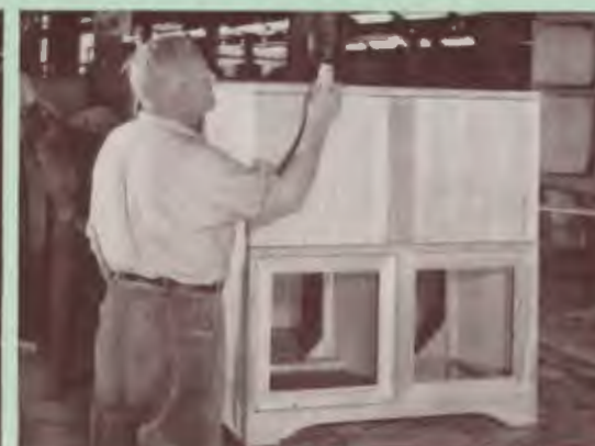
Meticulous hand sanding smooths edges, prepares the cabinet for the application of quality filler, stains and high gloss finish.
