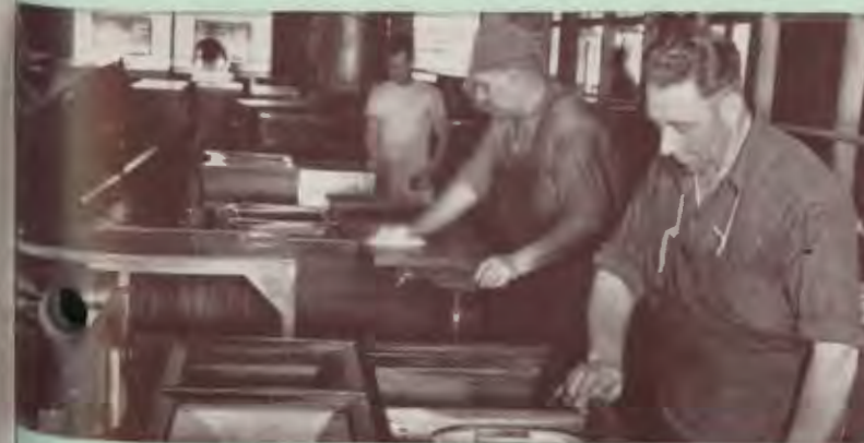
The lasting high gloss is the result of repeated hand-polishing done gently and precisely under constant, careful supervision.
