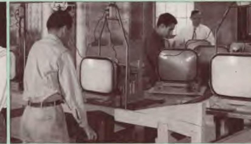
"LIVE POWER" TEST uses repeated 130 volt power surges to show up short-life parts so they may be replaced with parts that can be depended on for longer performance.
