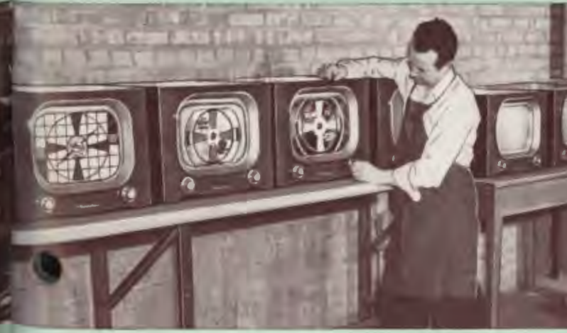
SPOT CHECKING pulls sets off the final assembly line at random and submits the chassis to a special inspection of power, reception, volume, tuning...other operational functions.
