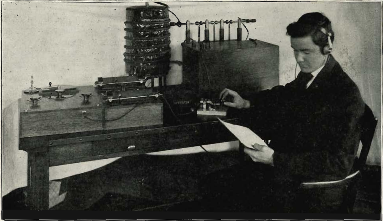
TYPE OF CLARK WIRELESS TELEGRAPH APPARATUS IN USE ON GREAT LAKE STEAMSHIPS
