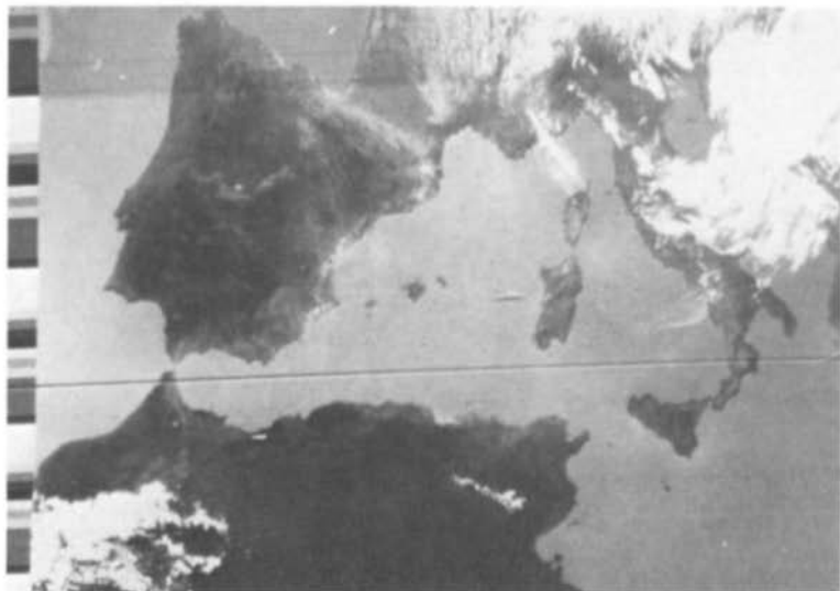
Fig. 91: An infrared image from TIROS-N (137.620 MHz). This shows that it is just as hot (dark) in Spain and Sicily as in Algeria and Tunisia. This satellite ceased operation on 1.11.80, and has been re- placed by NOAA 7 which is operating on the same frequency
