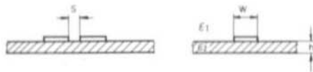
Fig. 1: Striplines in inhomogeneous medium (microstriplines). Left: Single line; Right: Coupled lines with \epsilon_{r\text{eff}} = K_{\text{EFF}} = \sqrt{K_{\text{EFFE}} \times K_{\text{EFFO}}}
