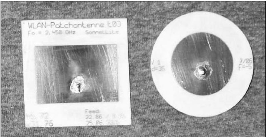
Fig 2: On the left is a rectangular patch antenna with an SMA connector for the feed. On the right is a circular patch antenna with an SMA connector for the feed.
