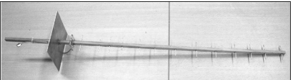
Fig 22: The 15 element Quagi for 2.4GHz with a plate reflector, it is 59.5cm long.
