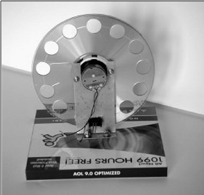
Fig 19: Light chopper using a CD and CD player motor.
