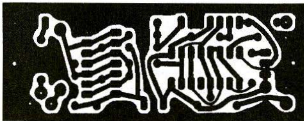
Fig.24: Supply Switch Interface PCB (single-sided 1.6mm glass-fibre-epoxy)
