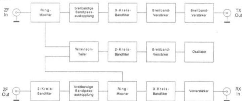
Fig.2: Block Diagram of the Universal Transverter
