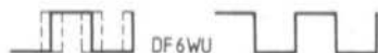
Fig. 3: The output voltage waveform at pin 3 (8) of the 7400. Left: wrong, right: correct working point adjustment
