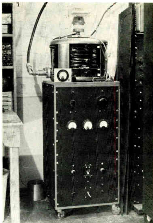
W6NLZ's modest 1 KW rig for 1296 mc./s. That's the bias battery at the top, field coil (all 4,000 turns) is rather noticeable. Eimac 3K2500 series operates the modest final. Which surplus yard did you find this in John?
