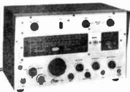
Two Unit Construction with Remote Modulator and Power Supply Conserves Space at Operating Position
