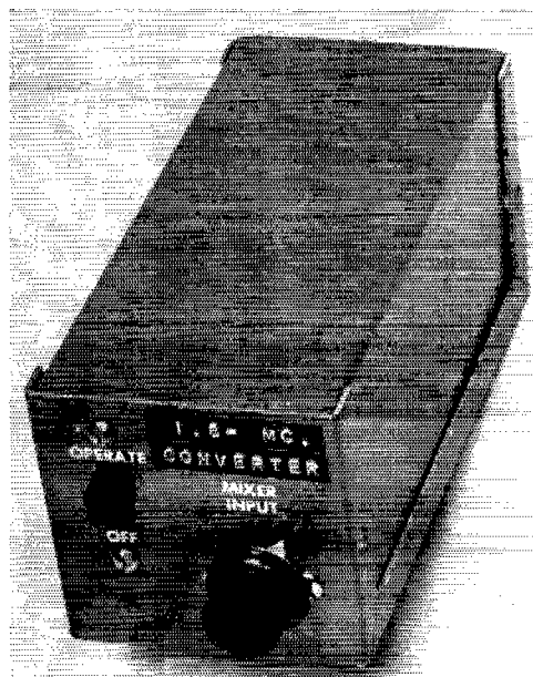
Top-front view of the converter showing the location of the on-off switch and the input peaking control. Input and output jacks are on the rear and bottom sides of the 2\frac{1}{4} \times 2\frac{1}{4} \times 5 -inch Minibox.
