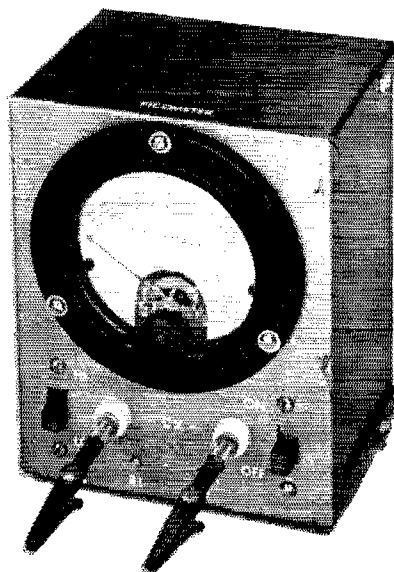
The completed Picometer which will test capacitor values from 10-pf. to 0.01- \mu f. Below the meter are the range switch, the clips to hold the capacitor under test, and the power switch. Below the clips are the two range adjustments.
