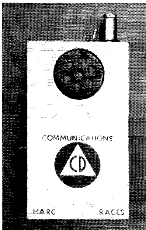
Fig. 1—A complete 50-Mc. transceiver, antenna and all in a 3 \times 5 \times 1 \frac{1}{4} -inch case. Whip extends to 52 inches total, giving good range with only a 9-volt battery for power.
