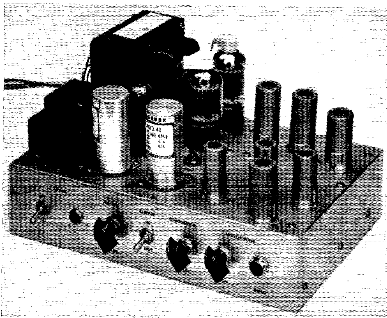
The de luxe modulator includes a speech compressor and a clipper-filter, along with a power supply that takes care of everything except the modulator plates. Miniature tubes, going from right to left, are: front row, 6AN8-A speech amplifier, 6AL5 compressor rectifier; second row, 6DT6-A compressor amplifiers; back row, 12AU7-A clipper, 6CG7 compressor driver and final voltage amplifier, 6CG7 driver. The 6GW6 modulators and modulation transformer are at the rear left; the components at front left are for the power supply. The multisection capacitor on the chassis above the clipper switch contains the three filter capacitors in the speech-amplifier section.
