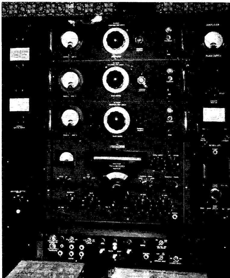
The operating position at K9LKA showing linear amplifiers for 10, 15 and 20 meters mounted in a rack above the receiver
