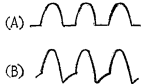
Fig. 3—Waveforms present (A) at the junction of R_3 and R_4 , and (B) after passing through differentiator C_3 - R_5 .
