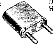
H-17T (HC-13/U). Pin Dia. .050". Pin Spacing .486". H-17TL (HC-13/U Except .093" Pin Dia.)
