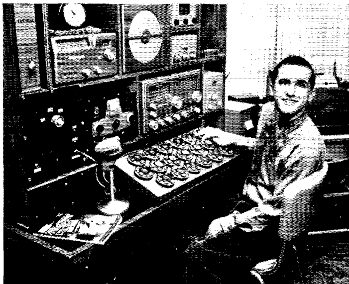
Terry Tatum, W6LKJ, and the nineteen telephone dials with which he is able to dial the code at about 12 w.p.m. Look for him on 40-meter c.w.
