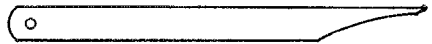
Fig. 5—An illustration of the unsoldering aid suggested by W7JJP. The tool is made from a hacksaw blade.
