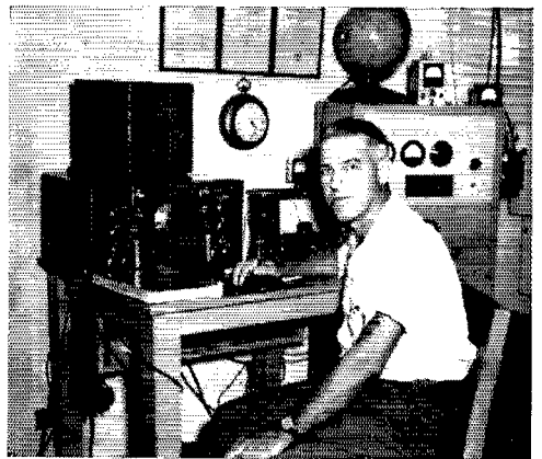
Lloyd D. McBurney, PJ2AF, with p.p. 807s in Class B modulating an 813, turned in South America's top 'phone tally, placed 7th among overseas 'phone entrants. Lloyd chatted with 412 W/VE contesters on 10, 15 and 20 meters.
