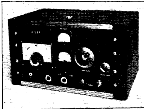
A front view of the 160-meter transmitter, showing the panel layout. The VFO is directly calibrated for 160 and 80 meters on the National SCN dial. The lower row of controls are, left to right, keying jack, buffer plate tuning, meter switch and the filament switch. To the right of the two meters are the final plate-tuning and the swinging-link controls.
