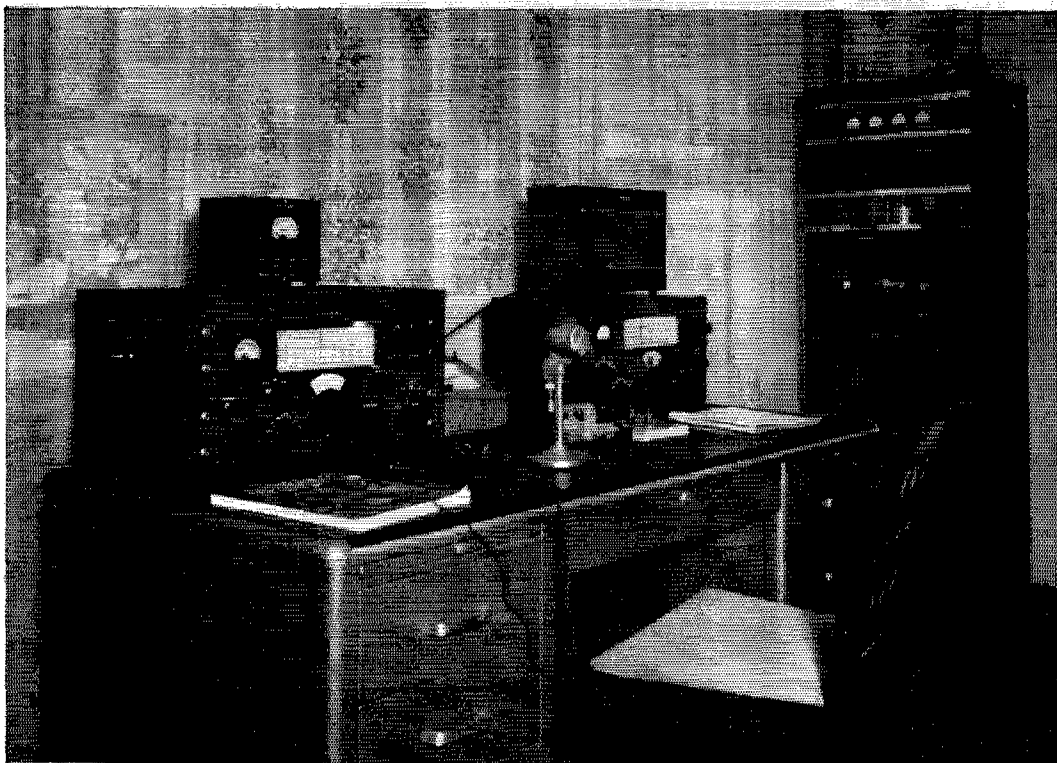
Left to right: Collins 75A-1 receiver, 310A-3 exciter with speaker above, 30K-1 transmitter
